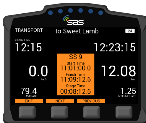
SCREEN 14. Times of completed stages
